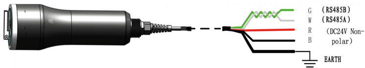
6.3 Diagram of wiring connection
