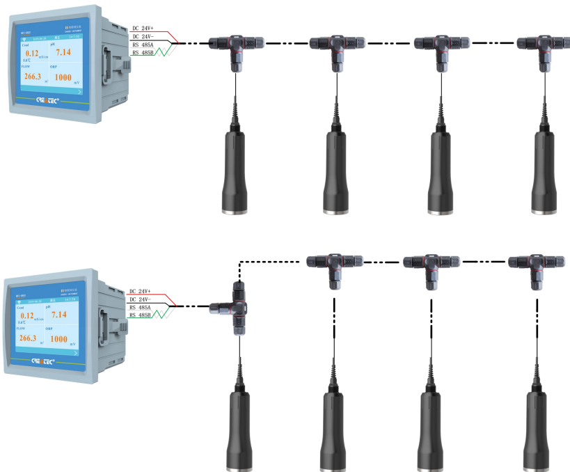
Figure 7.13 Field data bus serial application
